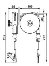
The balancer is fit with a device enabling to stop the stroke by carrying out a simple operation on the load.
