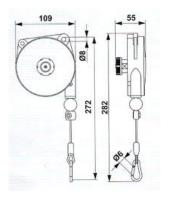
The balancer is fit with a device enabling to stop the stroke by carrying out a simple operation on the load.
